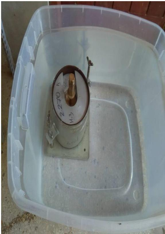
**Figura B7:** Probeta sumergida
